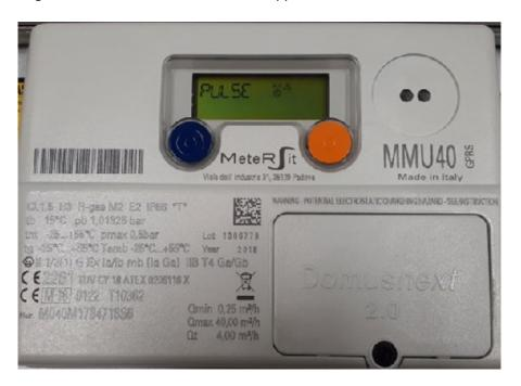
Keep pushing orange button for 7 seconds to activate Count pulse output: liters for pulse value appears (must be the same configure with MT Tool)
