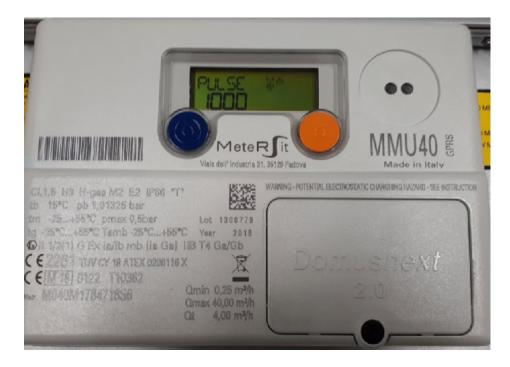
To disable pulse counter output keep pushing orange button on Pulse display until liters for pulse value disappears.
